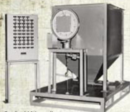
Cardinal 10-ingredient batching scale circa 1950.
